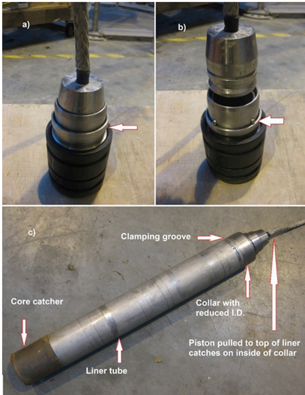
FIG. 3. (a) Assembled piston. Pushing down the outer sleeve (arrow) unlatches inner piston. (b) Outer sleeve is pushed down and ball bearings (arrow) are free to move outward, releasing the inner piston. Ball bearings also latch into the groove on the inside of the core chamber and are held out by an inner sleeve (just visible) that slides up on a spring as the inner piston is withdrawn. (c) Piston and liner assembled.
