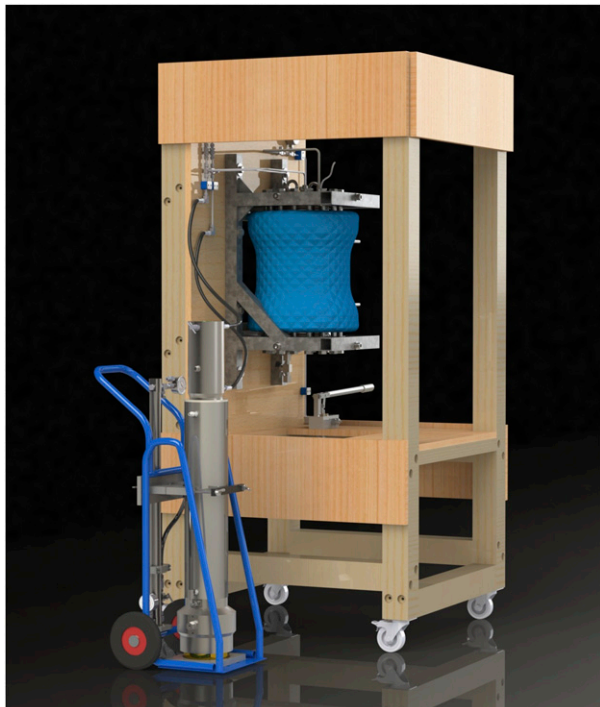
FIG. 10. Image of gill system connected to pressurized core chamber that has been removed from corer.
