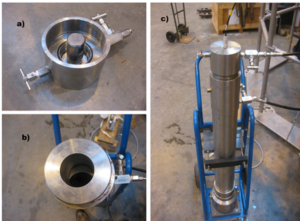
FIG. 2. (a) Top cap with optode fitted. (b) Top of core chamber showing ball valve half closed. (c) Top cap fitted and hoses to gill connected.
