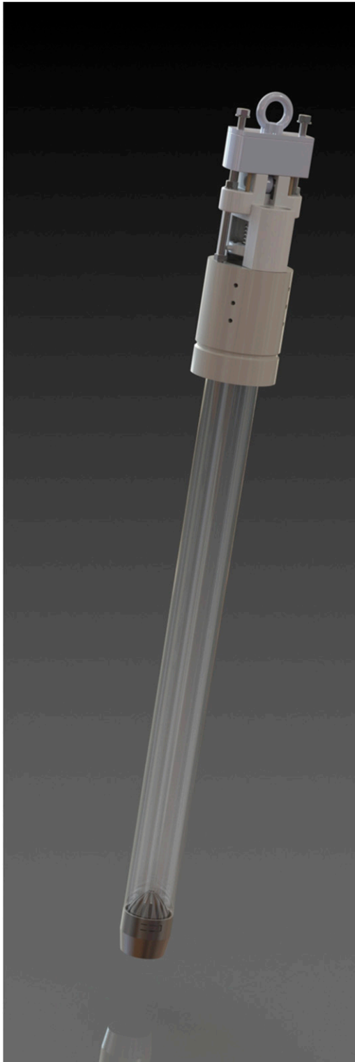
FIG. 7. Reference corer [computer-aided design (CAD) rendering].
