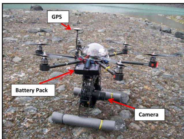
Figure 2. The hexacopter with key components labelled. [Colour figure can be viewed at wileyonlinelibrary.com ]
