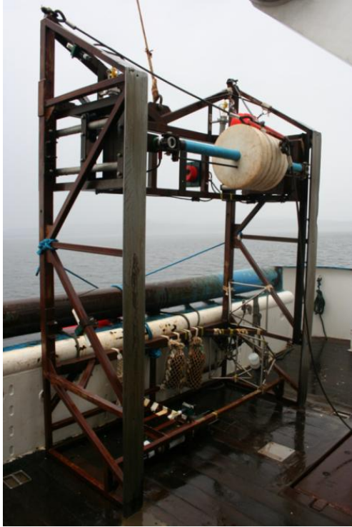
Figure 3 The towed sledge, sitting upright, used to tow the range of cylindrical objects supported on an axle.
