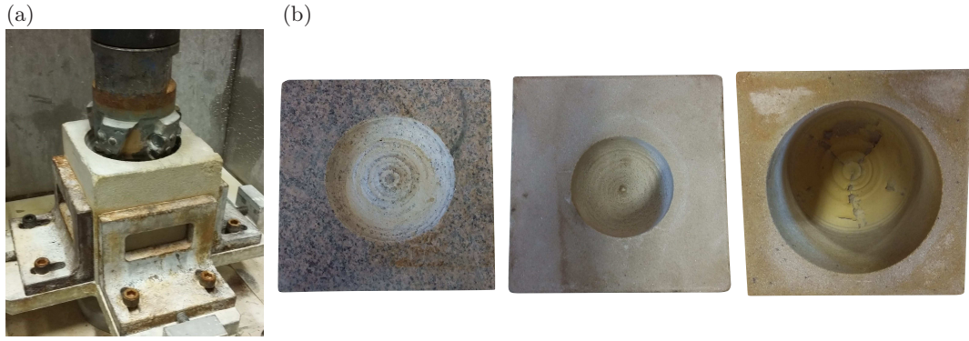
Figure 3: (a) A close up view on the drill-bit rock interface, (b) Examples of drilled granite and sandstone samples using various PDC drill-bits.
