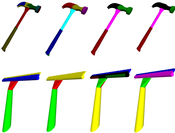
Figure 21. Various segmentation options for hammer and squeegee from ToolWeb: different colours represent different segments. For the hammer, left to right, we have a fixed number of clusters k = 5 and the smoothing parameter \lambda varying from \lambda = 0.1 to \lambda = 0.4 . For the squeegee, left to right, we have (k = 5, \lambda = 0.4) , (k = 5, \lambda = 0.5) , (k = 7, \lambda = 0.2) and (k = 7, \lambda = 0.3) .
