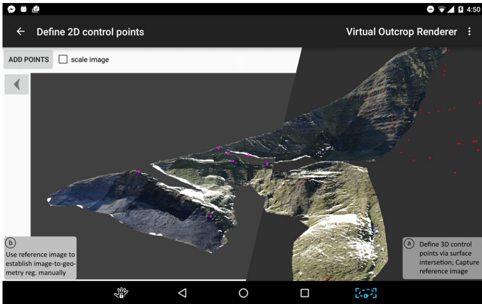
FIG. 7. The integrated 3D model viewer (“Virtual Outcrop Renderer”) of the framework allows defining 3D control points and capturing registration reference images (right, (a)). These reference images are used in a PnP -based manual registration process where the user selects 2D–2D point pairs (left, (b)).
