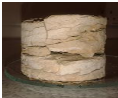
Figure 4: Damaged limestone due to treatment with ATMP.
