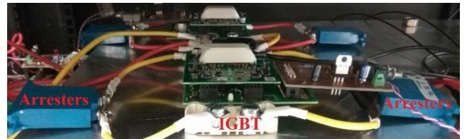
(a) The IGBTs and the arresters in the main breaker path
