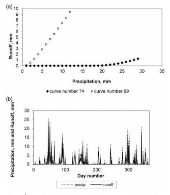
Figure 5 (a) Runoff against increasing precipitation at permanent wilting point for Halstow series soil, curve no. = 74; at field capacity, curve no. = 99. (b) Precipitation and runoff (in mm) for Halstow series soil at field capacity (using a separate climate dataset for model calibration).
