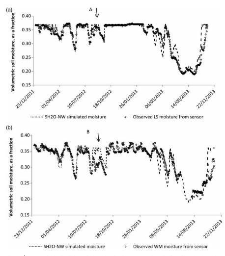
Figure 7 | SH<sub>2</sub>O-NW simulated and observed volumetric soil moisture (expressed as a fraction), also noting the portion of the graph (A and B) where observed sensor response varies between fields to multiple days of rainfall for (a) Longlands South and (b) Wyke Moor.
