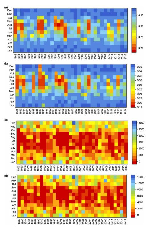
Figure 9 | Simulated volume moisture fraction 1982–2015 for (a) Longlands South and (b) Wyke Moor. Simulated runoff 1982–2015, m<sup>3</sup>/day for (c) Longlands South and (d) Wyke Moor.
