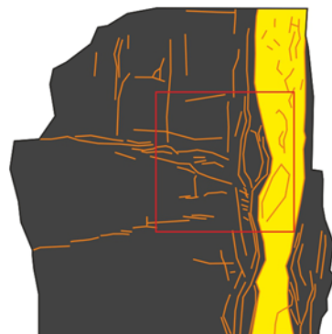
Fig. 4. Fe and Se laser ablation mapping of banded and cleat-filling pyrite in two Greenburn coal samples (map area depicted in schematic by red box). High Fe content defines all pyrite phases, while high Se concentrates in cleat-filling pyrite.
