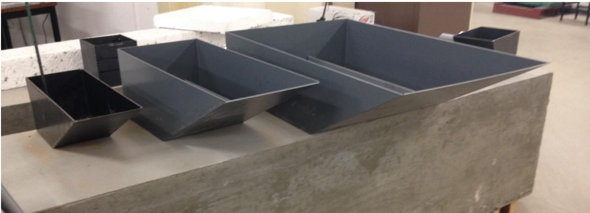
216 Figure 4. Scaled iceberg models with three different scour widths: 150 mm (steel), 250 mm (PVC) and 500 mm 217 (PVC). The rake angle for the three models is \alpha = 150^\circ .
