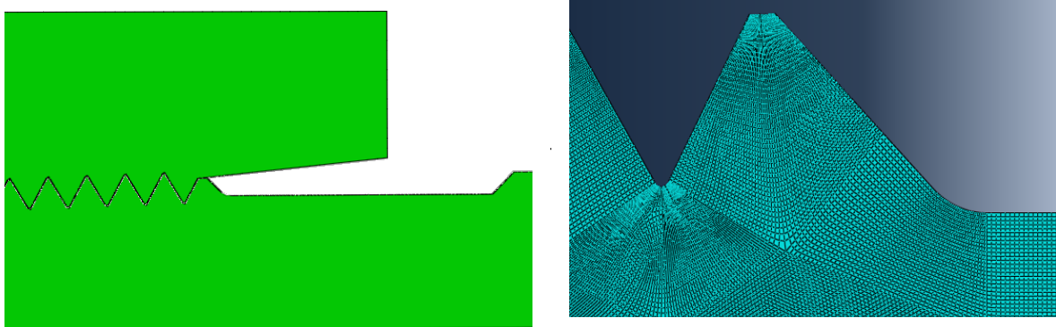
Figure 3 (left) FEA geometry (right) Mesh profile for LET and SRG
