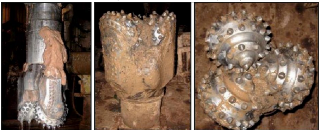
777 Fig. 9. Examples of bit balling of a tricone drill bit. Images courtesy of John Jong & Jon Royds, JX 778 Nippon Oil & Gas Exploration.
