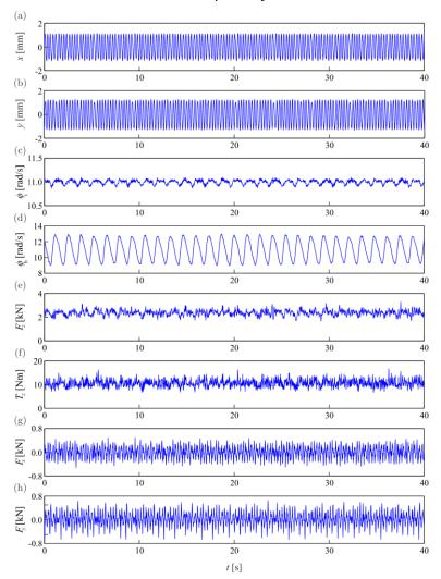
**Figure 3.** A sample of the recorded experimental time histories for configuration with 20 disks; (a) and (b) displacement of the BHA in the x and y direction respectively, (c) and (d) top and bottom speed, (e)  $F_z$ , (f)  $T_z$ , (g) and (h) transverse forces on x and y direction acting on the drill-bit.
