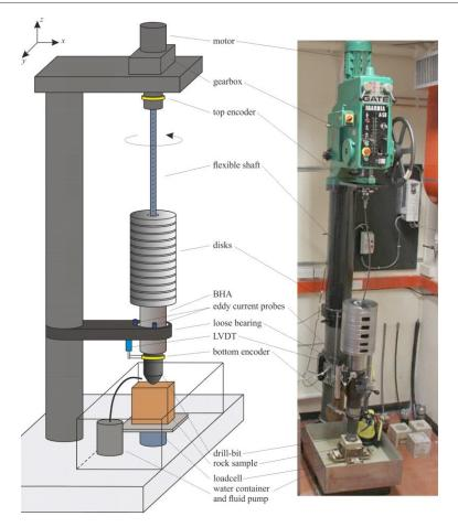
**Figure 3.** A schematic (left) and photograph (right) of the Aberdeen Drill-String Dynamics Experimental Rig showing its main components such as BHA, flexible shaft, WOB disks, drill-bit, rock sample and motor. The instrumentation include a 4D load-cell, LVDT, top and bottom encoders and eddy current probes.
