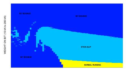
ROTARY SPEED (10 rpm to 150 rpm)
