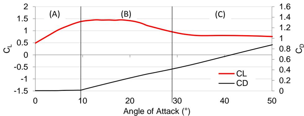
Figure 6-Lift and drag coefficient of the aerofoil NACA 64-618
