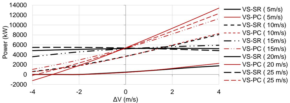
Figure 5- Comparison between the aerodynamic sensitivity of the VS-PC and the VS-SR wind turbines
