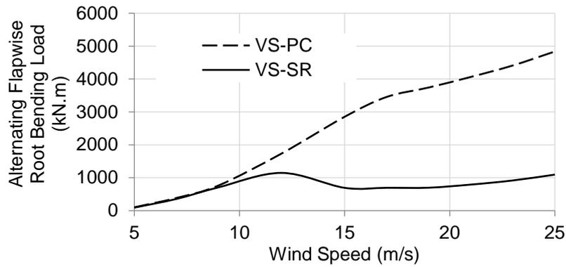
Figure 9-Comparison between the magnitudes of the cyclic (alternating) component of the root bending moment of the two wind turbines
