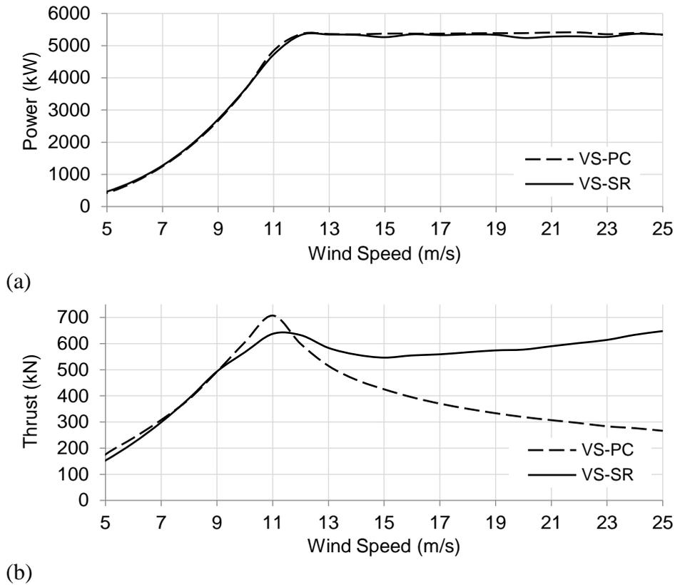
Figure 4-Comparison between the VS-PC and VS-SR power and thrust curves
