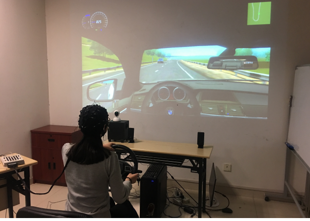
Figure 1. (Color online) The simulating experimental setup for obtaining EEG signals of subjects under alert and fatigue driving states.
