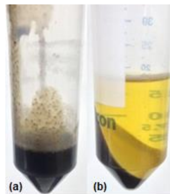
Fig 7. The mixture of rice husk and products after the reaction, using: (a) MnCl 2 ·H 2 O and (b) MnOx/Hi_ZSM-5 as a catalyst
