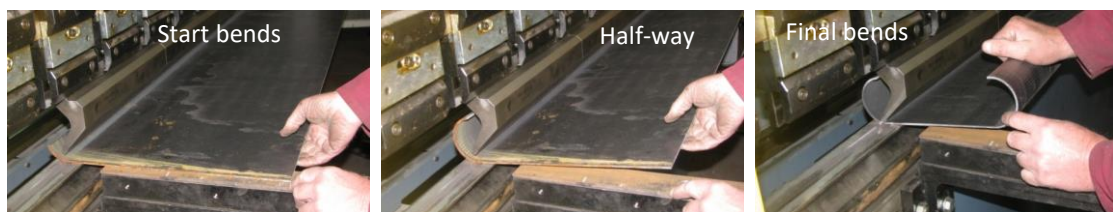
Figure 2. CFS joints with SB and CB bolting and F, S, S* and C types of beam sections and manufacturing process of a C section using a press brake.
