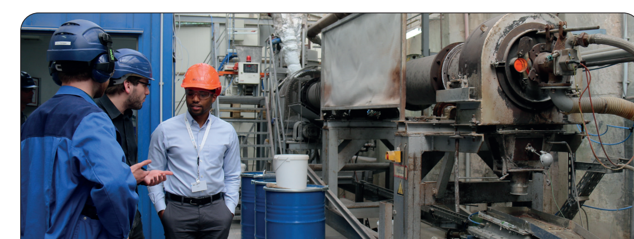
Figure 1: The KDO kiln at IBU-Tec AG was used for the pilot trial series.
