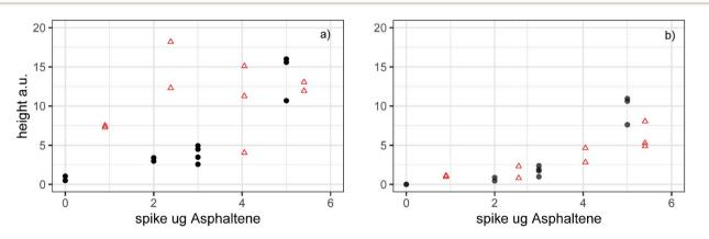
**Fig. 5** Comparison between the detector response (peak height) for (a) measured surface enhanced Raman spectra and (b) the surface enhanced Raman spectra corrected for the relative contribution of asphaltene, humic organic matter and pigments (height attributable to the G-peak at 1599 cm<sup>-1</sup>). Triangles = samples spiked with asphaltic petroleum, circles = tar sand.
