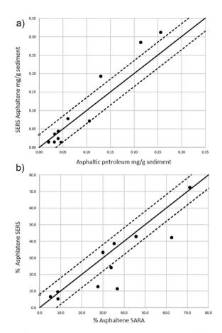
**Fig. 6** Graphical comparison between standard and SERS-based methods of analysing asphaltene and asphalt. (a) Comparison between ASTM D2414 and SERS based assay, and (b) between a total extraction-based quantification of bitumen content (ASTM D2172/D2172M-17e1) and SERS quantification of bitumen per gram of sediment. Dashed lines show 10% margins.
