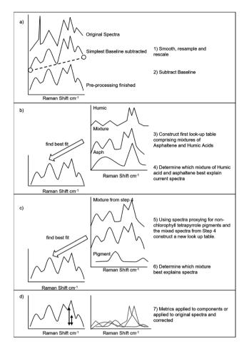
**Fig. 2** Algorithm used to deconvolve the components of a surface enhanced Raman spectra using look-up tables and entire spectra. (a) During pre-processing the data is smoothed, resampled to set resolution and a baseline subtracted. (b) The mixture of asphaltene and humic organic matter is determined. (c) The mixture of pigment and humic and asphaltic organic matter determined. (d) Metrics returned and quantification performed.
