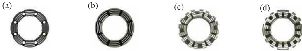
Figure 1: Coring bit profiles: (a) face discharge, (b) extended channel flushing, (c) V profile and (d) jet profile. Taken from [38]
