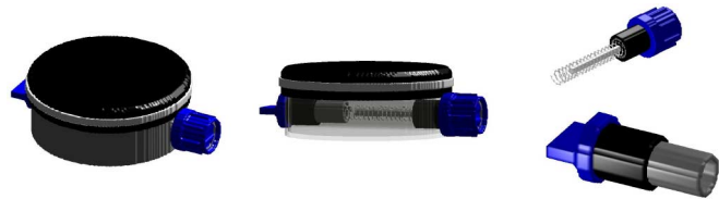
Fig. 10. Modeled AP landmine PMN. The adapted side parts of the landmine are shown at the right of the image. The black top of the AP landmine is rubber ( \epsilon = 6 ), the black pieces on the adapted parts is bakelite ( \epsilon = 3.5 ), shiny gray is perfect conductor (PEC), blue is plastic ( \epsilon = 3 ), the gray parts of the landmine are also bakelite ( \epsilon = 3.5 ), and the inside of the landmine is rubber ( \epsilon = 6 ).
