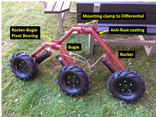
Fig. 9. Rocker-bogie with anti-rust paint. The second layer of paint was sprayed upon the anti-rust coating to improve the shelf life of the Rover Rocker-Bogie.
