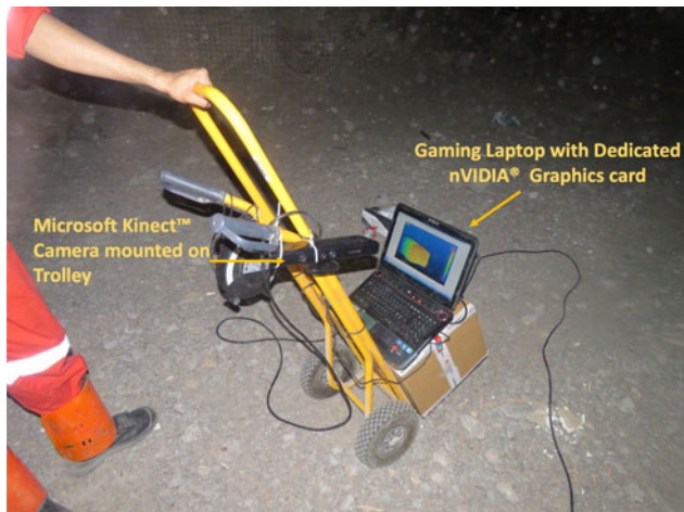
Fig. 3. InXSpace 3D system operated on a trolley during the MINAR5 campaign.
