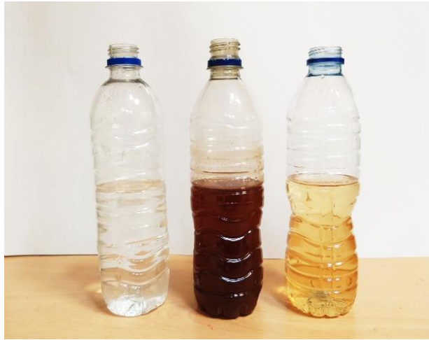
Fig. 6. Change in colour of water: before start of treatment (left) after hot-water/alkali-treatment (middle) and silane treatment (right) of OPBF
