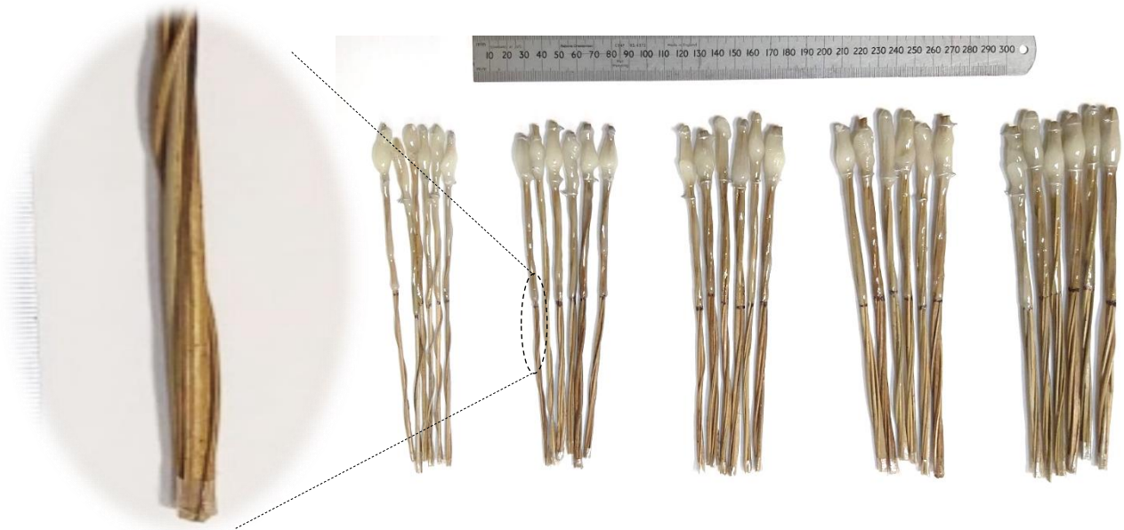
Figure 2.2: Illustration of OPBF tendons consisting of (from left to right) 2, 3, 4, 5 and 6 fibres per tendon respectively
