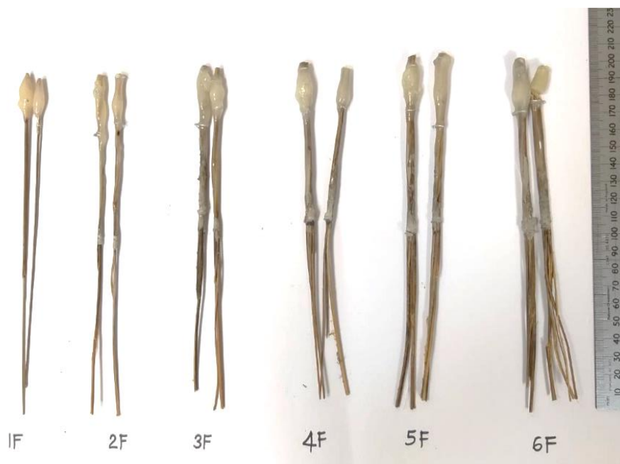
Figure 3.2: Illustration of damage to OPBF after complete pull-out at 112 days
