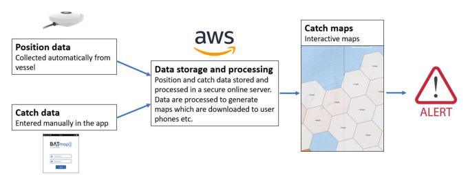
Figure 1: Overview of RTR as achieved by BATmap. See Figure 2 for a representation of the alerting system.
