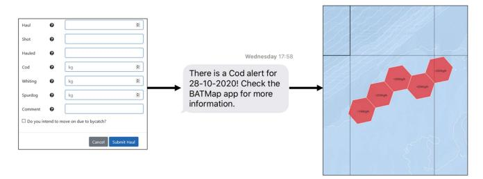
**Figure 2**: Schematic representation of the alerting system. The catch data is entered for each haul in the "Haul" tab. If the catch exceeds the ATV then it automatically triggers a SMS message to be sent. An SMS message prompts the user to open the BATmap app where the most recent alert is automatically displayed.
