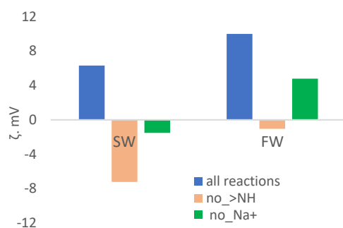
Figure 12: effects of >NH and Na + surface reactions on oil-brine \zeta -potential at 25°C.
