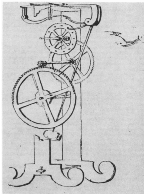
Figure 5: Pendulum clock conceived by Galileo Galilei around 1637. The earliest known pendulum clock design, it was never completed.
