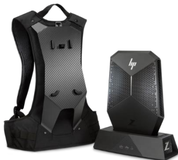
Figure 2. Illustrates HP Z VR backpack computer and docking station.
