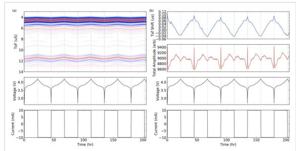
Figure 10. (a) Representative ultrasonic signal during cycling for several cycles of a lithium—cobalt oxide pouch cell at a C/20 charge/discharge rate. The ToF heat map shows maximum and minimum waveform amplitudes in red and blue, respectively. (b) Same ultrasonic data reduced to a ToF and amplitude metric. The blue and red lines represent the single ToF shift and amplitude measures, respectively. Reproduced from [74]. © IOP Publishing Ltd. CC BY 3.0.
