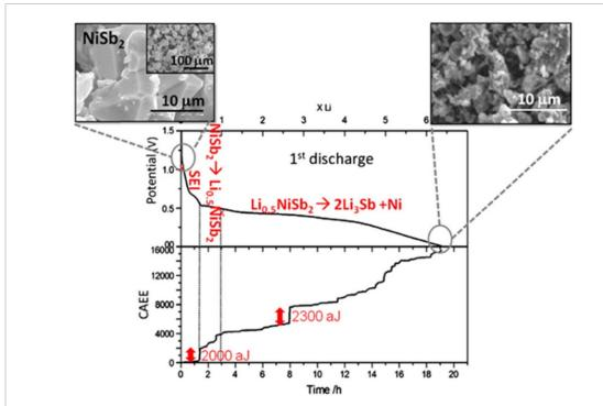
**Figure 6.** CAEE and voltage profile of the first discharge of the NiSb<sub>2</sub>/Li cell vs time (h), cycled at a C/10 rate between 1.5 and 0.0 V. Left inset: SEM image of the starting NiSb<sub>2</sub> powder. Right inset: NiSb<sub>2</sub>-based electrode after a full discharge [94]. Reprinted from [94], Copyright (2010), with permission from Elsevier.
