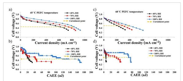
**Figure 16.** Correlation of PEMFC performance with acoustic activity. Top row: polarisation curve at 40%, 70% and 100% reactant RH, at 45 °C and 60 °C cell temperature respectively. Bottom row: corresponding acoustic emission CAEE at the various operating conditions. Reprinted from [30], Copyright (2019), with permission from Elsevier.
