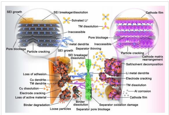
Figure 5. Outline of the most common degradation mechanisms in LIBs highlighting the highly complex and interconnected nature of the degradation phenomena in a cell.
