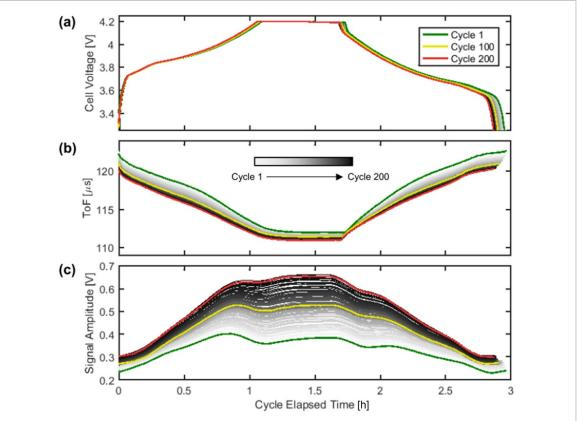
**Figure 12.** Cycle-to-cycle evolution of (a) cell voltage (b) ToF, and (c) signal amplitude, due to electrochemical ageing shown in progressive shades of grey as a function of cycle elapsed time. Data from the first cycle is indicated in green, the 100th cycle in yellow, and the 200th cycle in red. Reproduced with permission from [113].
