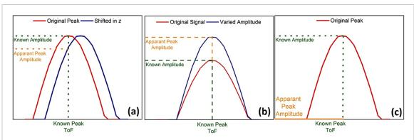
**Figure 4.** Typical amplitude variations in ultrasonic analysis including (a) amplitude shift due to shift in interface along the material thickness, (b) a measured increase in signal amplitude due to a higher acoustic impedance mismatch at a given interface and (c) the complete absence of the interface being measured due to the presence of a non-acoustically conductive layer [77]. Reproduced from [77]. © IOP Publishing Ltd. CC BY 3.0.
