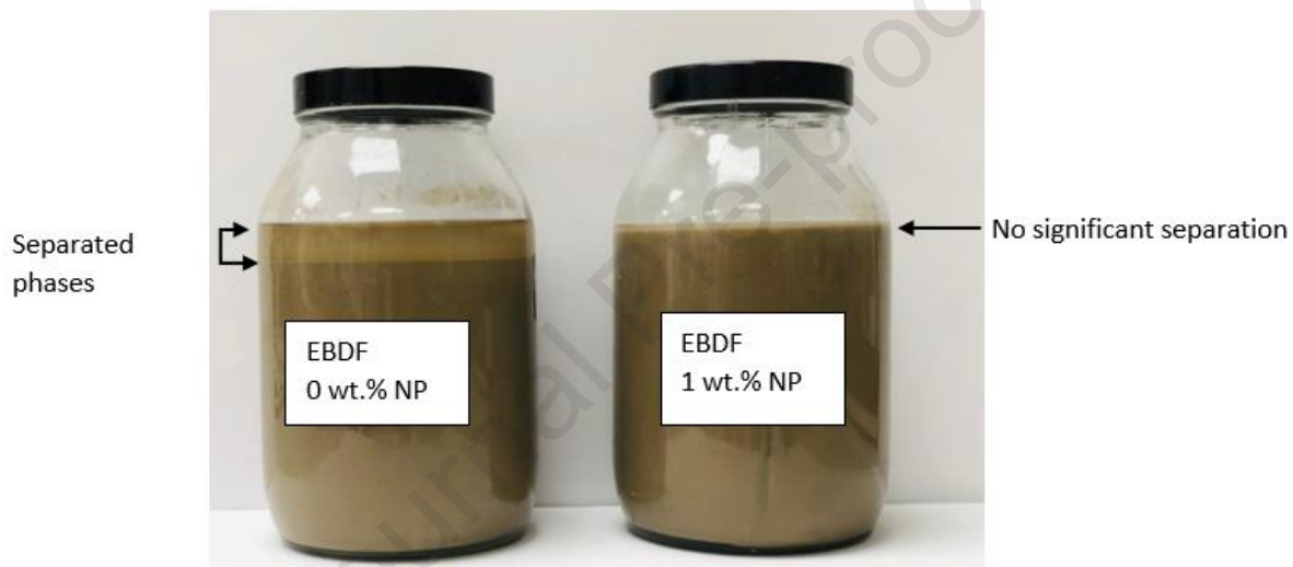
Figure 14: Stability of the base EBDF (left) and nano-enhanced EBDF with 1 wt% NPs sample (right) after 16 hr of static aging at ambient conditions.
