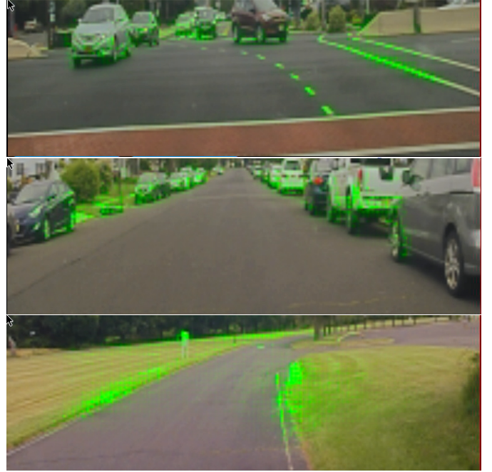
Fig. 1. Visualisation of Internal State of End-to-End System from [20]. Salient parts of input images were recovered using visual backpropagation. Green areas are highlighting these salient regions. As can be seen from the image, the model clearly learns to place high importance on relevant regions of images such as curbs and other vehicles.
