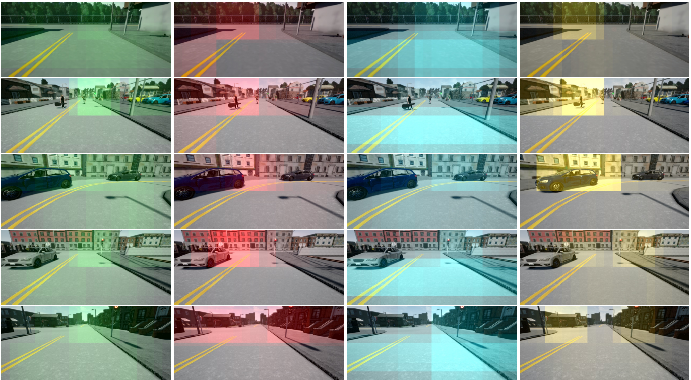
Fig. 2. Examples of attention maps for each high-level command from [21]. Commands are Follow lane (Green), Turn Left (red), Turn right (cyan) and Go Straight (Yellow). The various regions of input images that are learnt by the model to be important for each command are highlighted in the images and can be output as shown to provide a level of explainability for the networks decisions.
