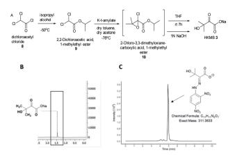
Fig. 2 (A) An optimised synthesis scheme towards HMKB 3 starting from dichloroacetyl chloride 8, *via* isopropyl 2-chloro-3,3-dimethyloxianoate 10 as a transit intermediate. (B) <sup>1</sup>H-NMR of 3 confirming the presence of the compound. (C) Extracted ion chromatogram (EICs) from LC-MS analysis of 3-DNPH.
