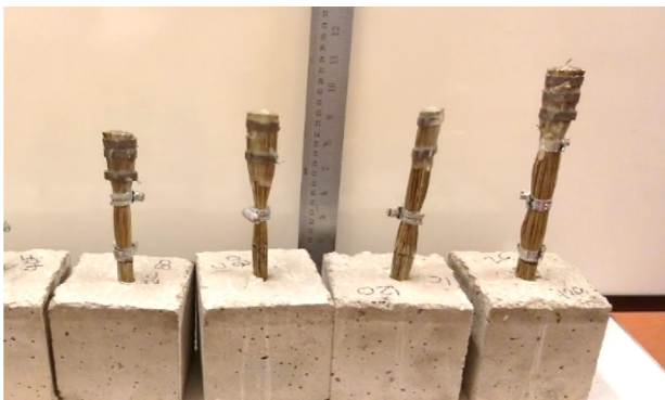
Fig. 9. Some bond pull-out samples showing strand pull-out from concrete matrix.
