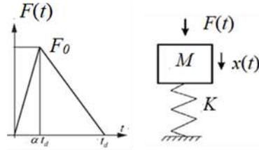
**Fig. 1.** Unsymmetrical triangular pulse shape (left) system (right)
