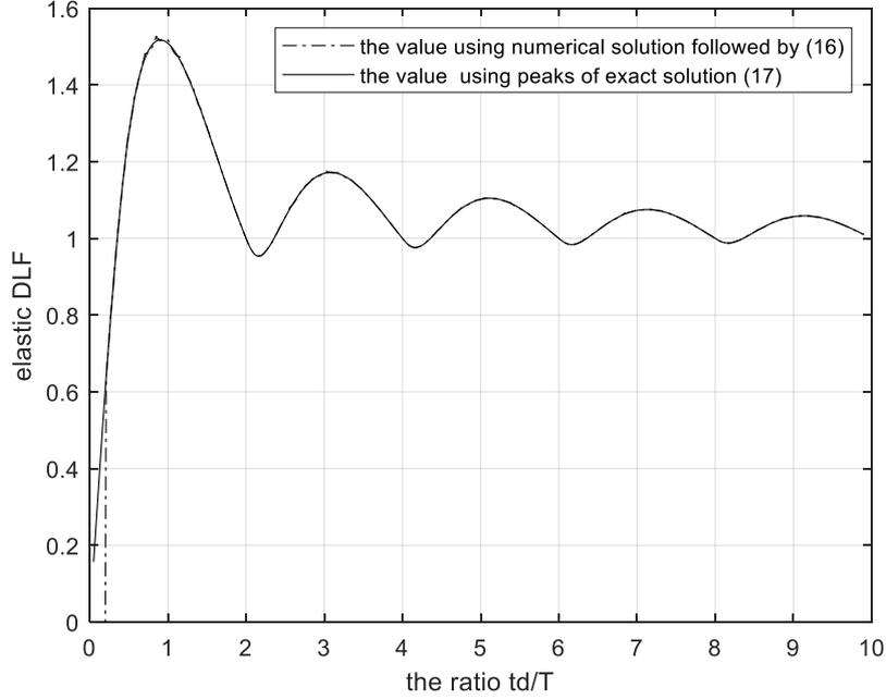
**Fig. 2.** Elastic DLF using Numerical and analytical method
