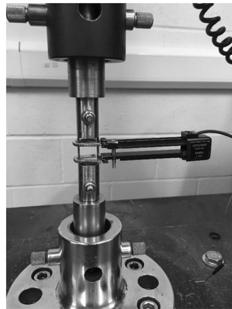
Fig. 7 Set-up of the column tensile coupon test
