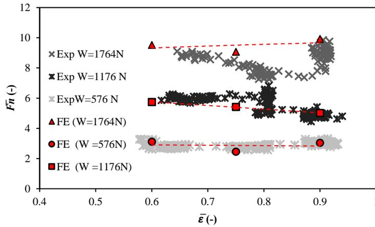
Figure 13: Experimental correlations for  $\bar{F}_n$  against  $\bar{\epsilon}$  for multiple discs of  $d=0.2$  m,  $t=0.025$  m and  $n=6$
