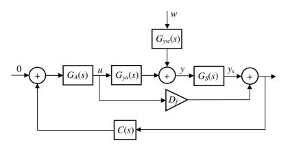
Figure 1: Positive-position feedback. General control scheme.
