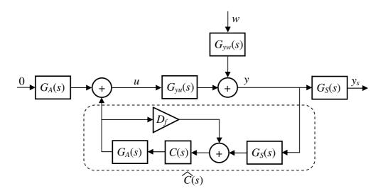
Figure 2: Equivalent representation of the general control scheme.
