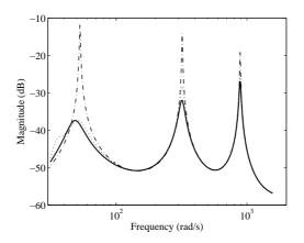
Figure 6: FRF of  $G_{zw}$  for the first three vibration modes.  $(-\cdot -)$  open-control, (-) closed-loop with C(s) of Eq. (30) for  $p_1 = 3$ ,  $D_f = -G_{yu}(0)/0.91$  and  $\gamma = 6.8 \cdot 10^3$  and (--) closed-loop with  $C(s) = \gamma/s$  for  $D_f \gamma = -226.2$  and  $1/D_f = -18$ .
