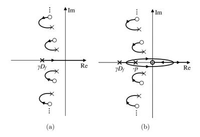
Figure 4: Design method proposed in [22]. (a) Pole-Zero diagram when  $C(s) = \gamma/s$ . (b) Pole-Zero diagram when  $C(s) = \gamma/s$  and  $G_S(s) = s/(s+p)$ .
