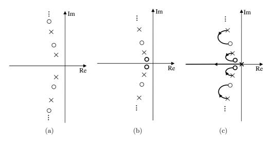
Figure 3: Design method proposed in [18]. (a) Pole-Zero diagram of  $G_{yu}(s)$ . (b) Pole-Zero diagram of  $G_{yu}(s) + D_f$ . (c) Root locus of  $(G_{yu}(s) + D_f)(\gamma/s)$ .
