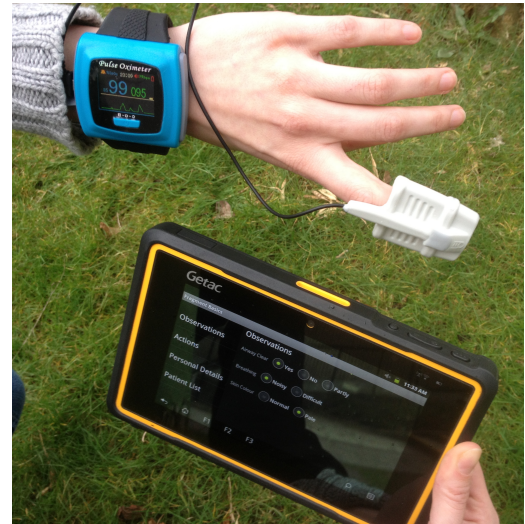
Figure 1: First hardware prototype (Getac Z710 tablet and Pulse Oximeter sensor).
