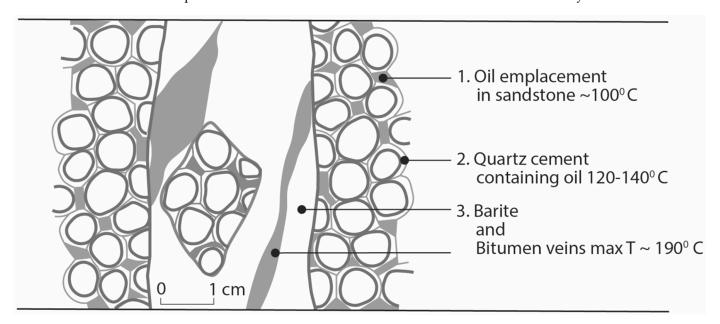
**Figure 9.** Schematic images of oil temperature history in sandstone, quartz cement and barite-bitumen hydrothermal veins.
