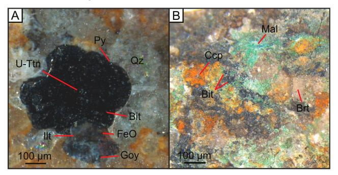
**Figure 4.** Optical microscopic images of **(A)** U-Ttn bearing bitumen nodule that fills sandstone porosity; **(B)** Cu-bearing, bitumen-barite vein that cuts sandstone country rock. Bit = Bitumen, U-Ttn = Uranium-titanate, Py = Pyrite, Qz = Quartz, FeO = Iron Oxide, Ilt = Illite, Goy = Goyazite, Brt = Barite, Ccp = Chalcopyrite, Mal = Malachite.
