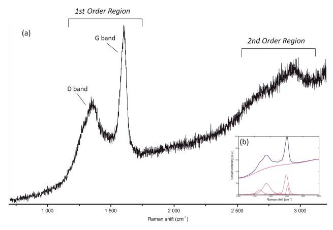
**Figure 5.** (a) Example of bitumen Raman spectra from hydrocarbon veins showing the presence of the D and G bands in the first order region and broad bands in the second order region; (b) example of the deconvolution using the IFORs software [42].
