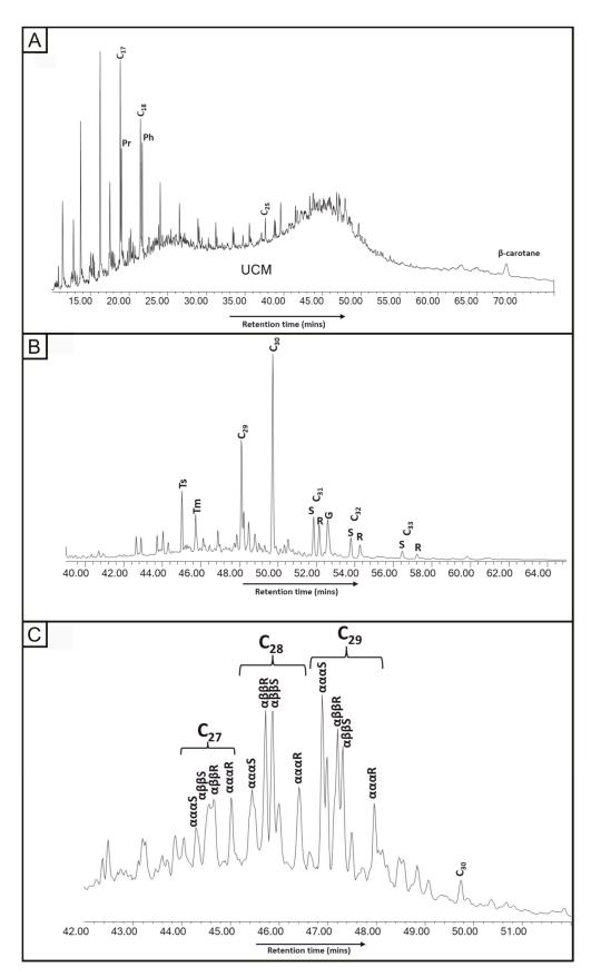
**Figure 6.** Mass chromatograms for oil residue in Yesnaby Sandstone. (**A**) m/z 85 n-alkane distribution with  $\beta$ -carotane (highlighted); (**B**) m/z 191 hopane distribution with gammacerane (highlighted); (**C**) m/z 217 sterane distribution.
