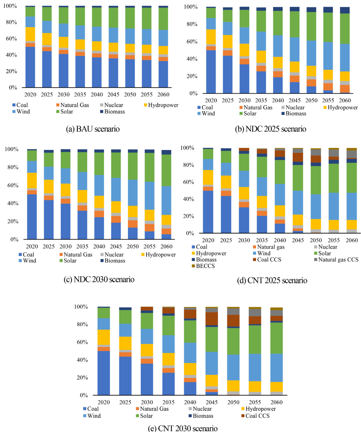
Fig. 6. Share of each technology in the total installed capacity under different scenarios.
