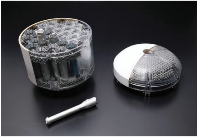
FIG. 4. This image shows a concept model of NASA's orbiting sample container, which would hold tubes of martian rock and soil samples that would be returned to Earth through a Mars sample return campaign. At right is the lid and a model of the sample-holding tube is shown at bottom left. The sample container would help keep contents at less than about 30°C to help preserve the Mars material in its most natural state. Photo Credit: NASA/JPL-Caltech.
