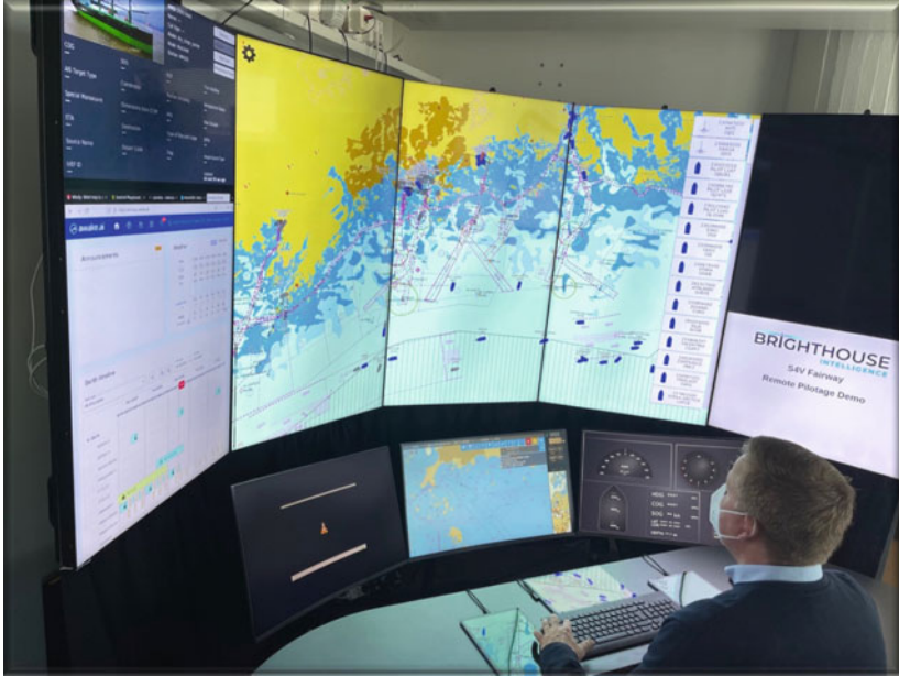
Fig. 2 From Aboa Mare—remote pilotage center ( Source Author)
