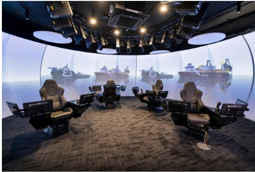
Fig. 3. View of the 300 deg toroidal dome (9 m diameter) visualisation suite of the NDC Marine Simulator. The system consists of 22 pcs (8 to run 16 projectors, 8 to run 4 control chairs and 6 to run the physics engine of the software). Assignable chairs are shown in the picture, which can control 2 vessels and 2 cranes/ROVs at the same time, therefore allowing for simulating operational scenarios involving simultaneous operation of these assets.
