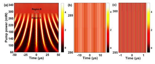
Fig. 6. (a) Progressive temporal evolution of pulse laser from PQS to QSML to CWML state; (b), (c) Zoomed-in pulse evolution in QSML (Region A) and CWML (Region B) operation states.
