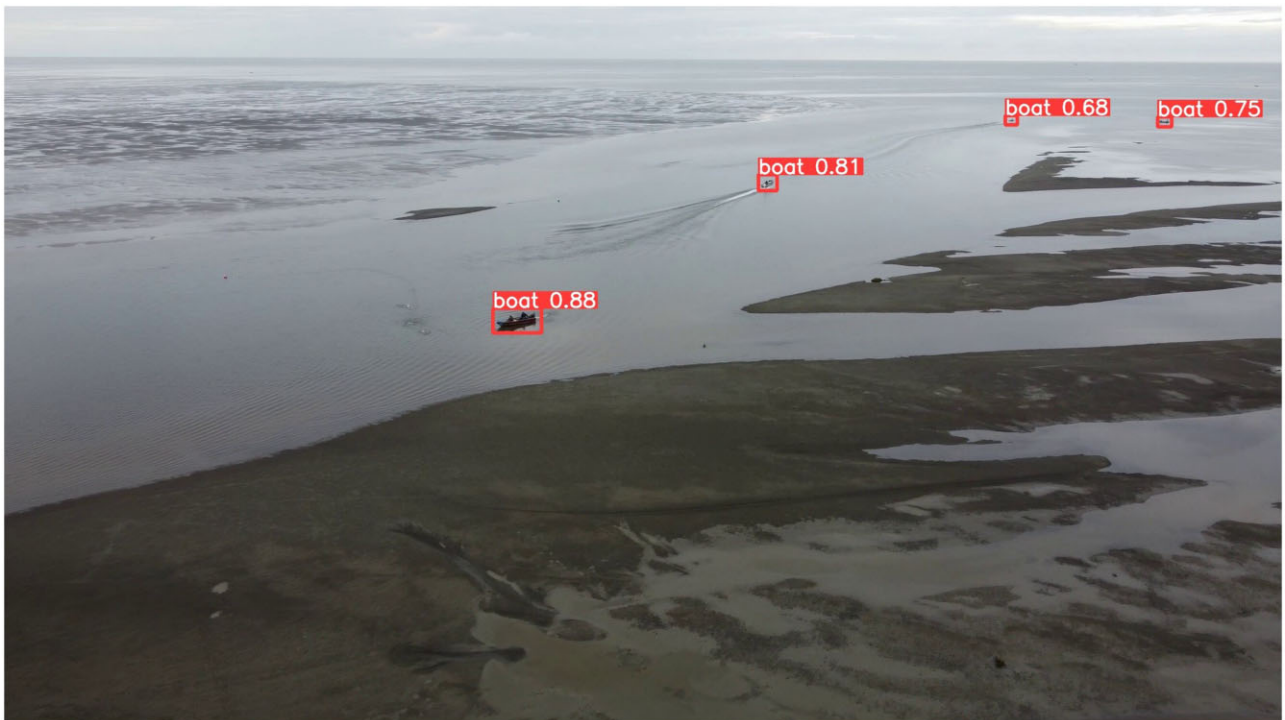
Figure 21. Object detection results on 2021 imagery collected from a test flight near Quinhagak. Image credits: Sean Gleason and Nalaquq, LLC (2022).
