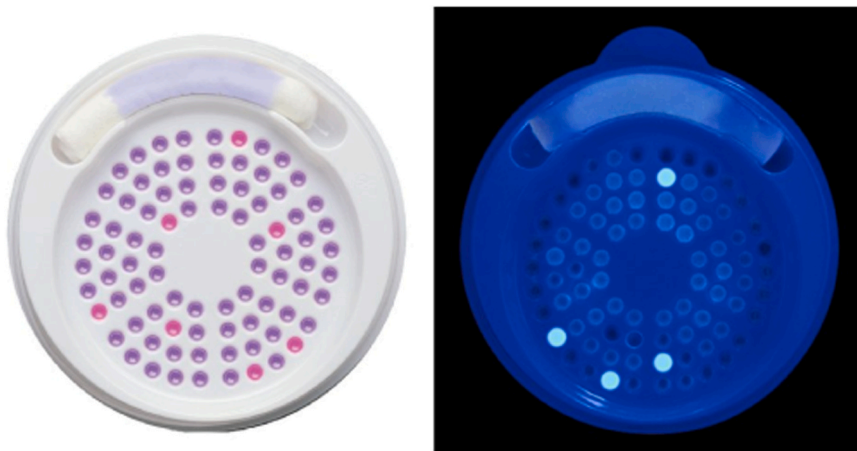
Fig. 3. SimPlate® system: (left) pink wells indicate a positive result for total coliforms [103]; (right) fluorescence in wells indicate a positive result for E. coli [104].
