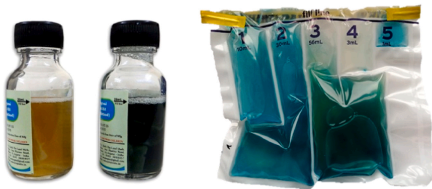
Fig. 1. (Left) Hydrogen sulfide (H 2 S) method. Field-testing vials manufactured and marketed by Water Health Laboratories under contract with UNICEF [58]. Yellow vessel indicates a negative result, while black vessel indicates a positive result. (Right) Aquagenx® Compartment Bag Test (CBT) for MPN. Pale yellow compartment indicates negative result, blue-green compartment indicates positive result for E. coli , and compartments that fluoresce blue under 365 nm UV light indicates positive for total coliforms.
