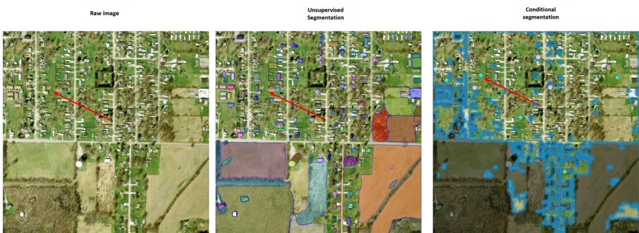
**Figure 28.** Schematic diagram of green space segmentation within the city. In general, when employing conditional green space extraction, it proves challenging to effectively extract green spaces in the presence of small buildings. Conversely, with unsupervised classification, the extraction of buildings is more successful. The red arrow points to the region we need to segment out.
