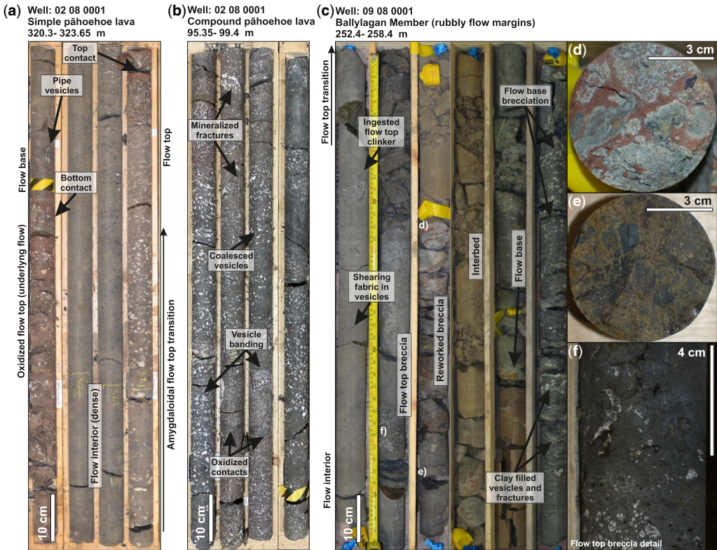
Fig. 9. Figure highlighting typical features of the Antrim lava pile as seen in NIRE borehole core. (a) Example of a simple pāhoehoe lava flow from within Lower Basalt Formation of the 02 08 0001 borehole showing typical asymmetrical vesicle distribution and oxidation towards the flow top. (b) Example of a compound pāhoehoe lava flow from within the Lower Basalt Formation of the 02 08 0001. (c) Details from the Ballylagan Member of the Interbasaltic Formation highlighting the presence of rubbly flow margins associated with flow margin autobrecciation. (d) Reworked and leached scoriaceous breccia clasts in oxidized matrix. (e) Reworked and deeply altered volcanoclastic breccia with scoriaceous clasts likely reworked from underlying rubbly flow top. (f) Detail of flow top breccia.
