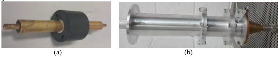
Fig. 1. Photos of axisymmetric system. (a) Ceramic tube around a bronze rod. (b) Coaxial structure with material under test inside.
