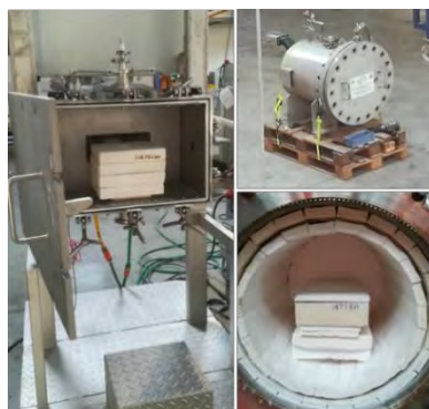
Fig. 2. The used MW equipment and set-ups in upscaled roasting experiments: MEAM Explorer VP 2 (left) and MEAM MP 6 (right).
