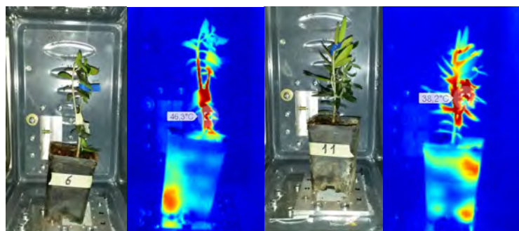
Fig. 4. Test with a custom 4-ports chamber at 2450MHz
