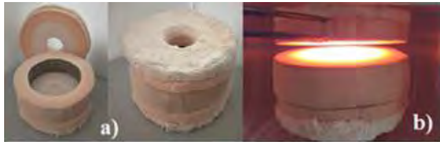
Figure 2: Sintering chamber: (a) at room temperature, (b) at the end of sintering test.
